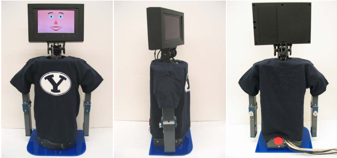
Figure 2. Picture of the front, side, and back view of Troy. Adapted from “Design and Evaluation of a Humanoid Robot for Autism Therapy,” by Daniel Ricks, 2010, Brigham Young University, Provo. Reprinted with permission.
